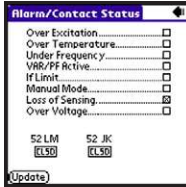
Figure 6-20. Alarm/contact Status Screen
