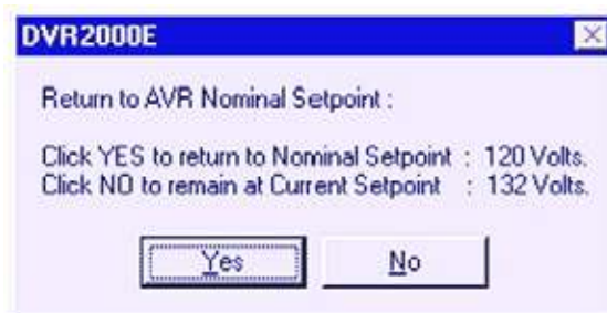
Figure 5-14. Message Box - Return to AVR Nominal Setpoint
